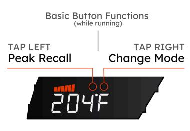
Pressing the peak recall button while on the O-60 timer will cycle through timers
